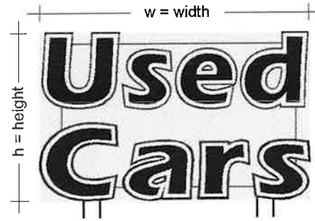
Calculating Area of a Sign where Copy Exceeds Sign Area = (height of copy) x (width of copy)
