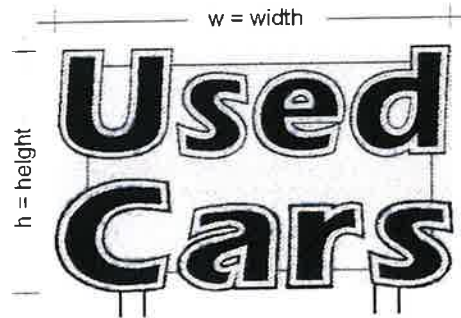
Calculating Area of a Sign where Copy Exceeds Sign Area = (height of copy) x (width of copy)
